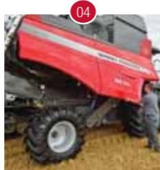
04 One piece panels allow for quick inspection access
