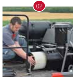
02 Checking and cleaning the air filter
