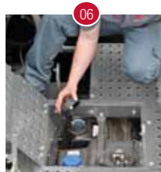
06 Easy refueling - both tanks are located next to each other for easy access
