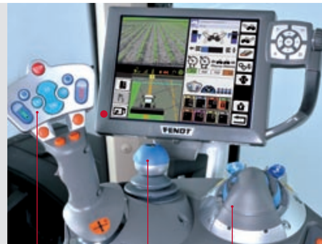
Multi-function joystick Controls Valve 3 and 4, power lift automatic mode
