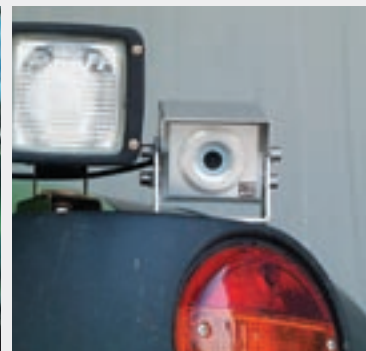
Camera for the Varioterminal
