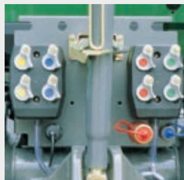
Double-sided connect-under-pressure couplings; external load sensing hydraulic connection
