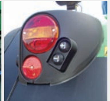
External control for hydraulic control unit at rear
