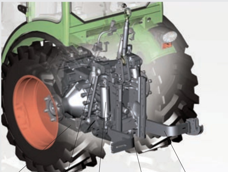
Power lift control on load-sensing pin Cylinder for tilt adjustment Lifting cylinder Cylinder for lateral adjustment Lower link
