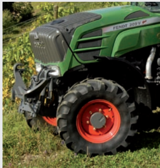
The lower links on the front power lift can be folded up without using tools.
