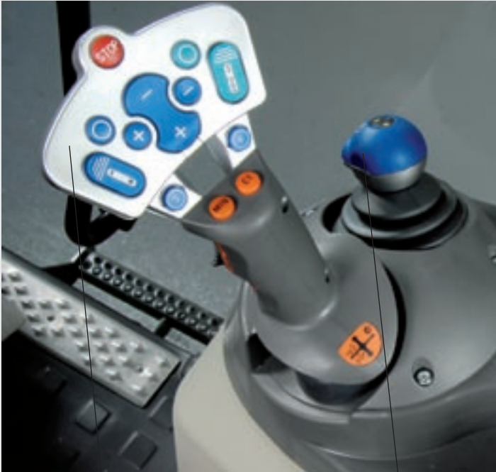
Multi-function joystick, with buttons for the rear power lift, control valves, 3rd and 4th electric circuit, cruise control and engine speed memory keys.
