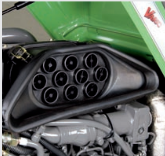
The air filter with cyclone pre-cleaner stands for maximum efficiency, despite the small installation space in compact tractors.
